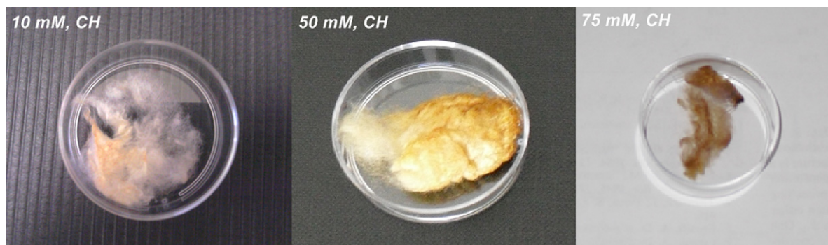
Fig. 3. Comparison of photographs showing fibers equipped with AgNPs by conventional heating (CH) using different AgNO 3 precursor concentrations.
